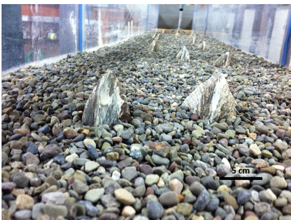
Fig. 2 Image of Lampsilis siliquoidea shells randomly placed in the experimental area of the flume to create a moderate density (10 mussel per \text{m}^2 ) mussel-covered bed
